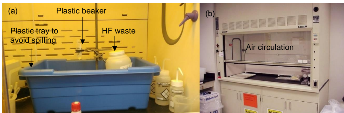
Fig. 3.14 (a) Equipment for metallographic etching and (b) fume-hood to perform HF etching.
